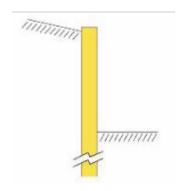
Secant pile walls are composed of both reinforced and non-reinforced piles. Typically, the non-reinforced piles are installed first and are made of cement/bentonite or low-strength concrete. Following this, the reinforced piles are placed, with the reinforcement consisting of either cages or I-beams.
